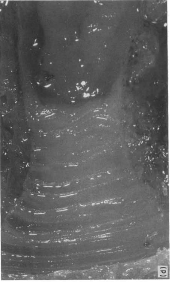
Figure 12 Photomicrographs obtained with the stereo optical microscope of the anterior annulus showing lamellar bulging and buckling. Magnification 35 \times . (a) With no load and (b to d) loaded to 0.20 compressive strain.
